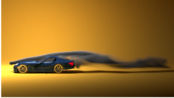
Figure 10: Side view of the 3-D wind-tunnel simulation shown in Figure 1. Note the vortices behind the car.
